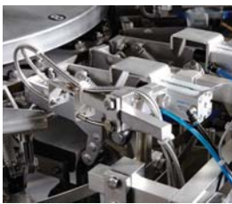
Pouch position & 2-sheet detection
